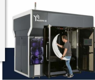
Operator removing a huge car bumper prototype from the Massivit 5000 3D printer (Source: Massivit)
