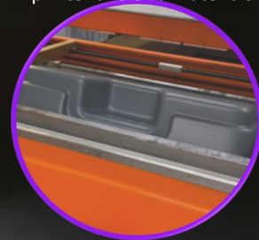
A thermoforming mold produced using a Massivit printer and Sika materials
