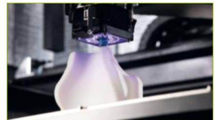
The Massivit 10000 introduces to market the first true isotropic 3D-printed mould for composite manufacturing
