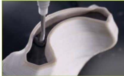
A detail of the "cast in motion" technology for the mould of a car roof
