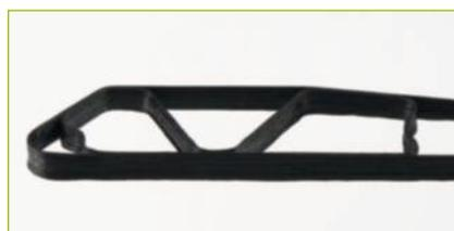
3D-printed truss made in continuous carbon fibre and epoxy resin
