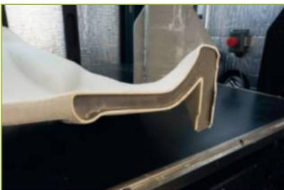
The Massivit 10000 3D's Cast In Motion (CIM) technology combines ultra-fast, additive manufacturing technology with high-performance, thermoset materials to enable automated tooling for composites
